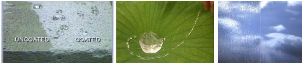
**Fig.6.** Self-cleaning coated surfaces
