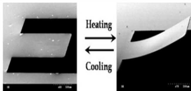
**Fig.4.** TiNi cantilever showing the actuation during heating and cooling
